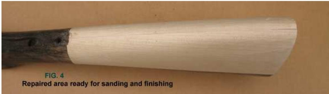
After the sawdust settles and the surfaces all faired-out and blended seamlessly, it’s time for finishing: “whiskering” and final sanding, staining, filling, and the oil and wax finishes. Everybody seems to have their own approach to these processes and enough has been printed in “how-to” gun books and past issues of **THE AMERICAN RIFLEMAN** so I won’t regurgitate any of that stuff here. Just a couple remarks on staining that aren’t adequately addressed in those sources:
